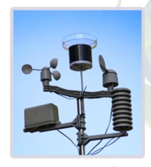
Over all Weather system consists of a The Integrated Sensor Suite (ISS) which comprises of
